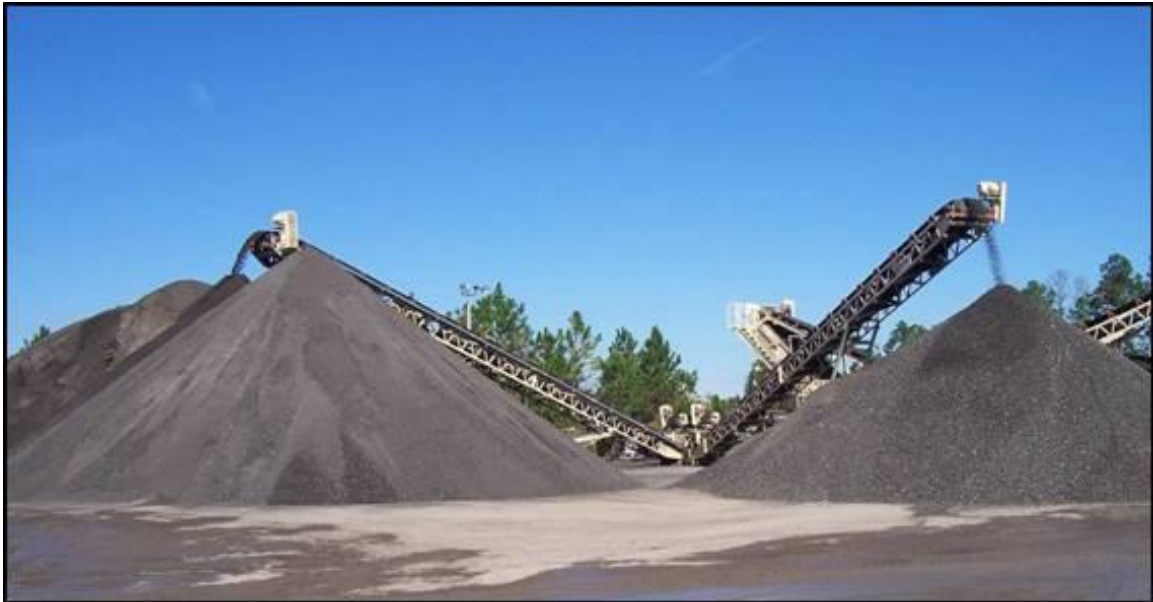
Figure 4-3 RAP Fractionation into Coarse FRAP (right) and Fine FRAP (left) Stockpiles
