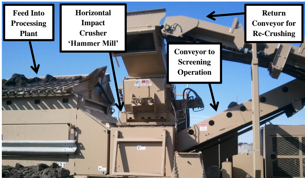
Figure 2-3: RAP Processing Equipment - Hammer Mill Crusher
