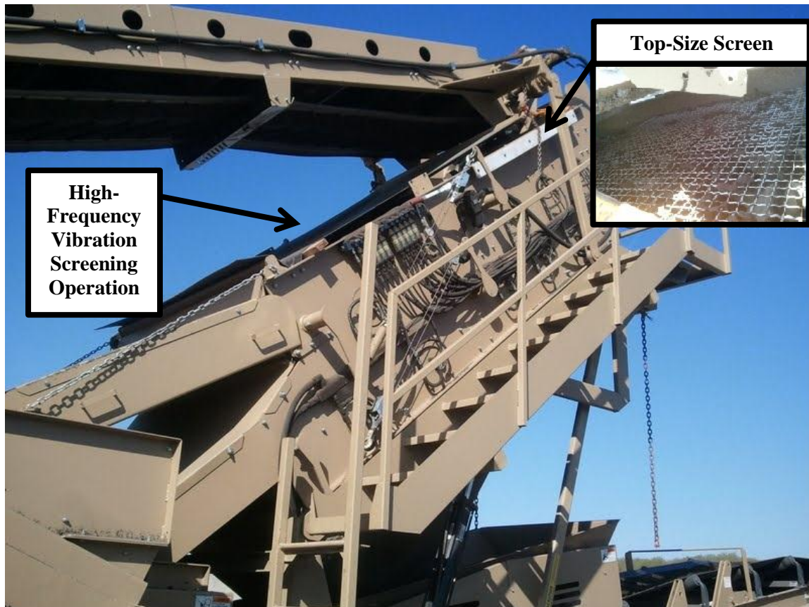
Figure 4-1: High-Frequency, Stacked-Screening Operation for Fine RAP Removal
